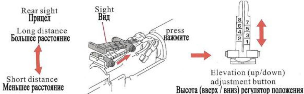
The AK series rear sight is a tangent type which is adjusted vertically according to distance to the target.
